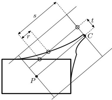
**Figure 8.** The general algorithm geometrically. The rectangle is to be connected, with the middle of the connector at  $C$  and the starting location inside the rectangle at  $P$ . The edge of the rectangle is displaced in the direction of  $PC$  according to Eq. (1). The angle of the rectangle is visible on the displaced curve.
