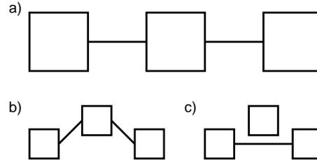
**Figure 1. An extreme example of the visual ambiguity inherent in complex boxes-and-lines diagrams when the layout is restricted: a) the ambiguous diagram, b), c) possible meanings. If the diagram was designed by a human, one can be certain that b) is the correct interpretation.**
