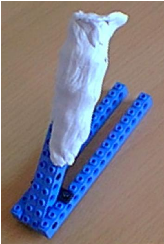
Figure 13. An ergonomic handle implemented using air-hardening modelling paste. The handle was molded directly to the left hand of one of our research group’s members.
