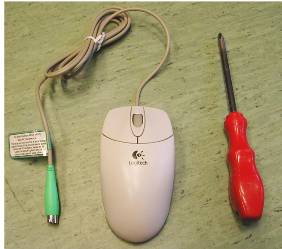
Figure 1. The non-LEGO parts and tools required for a controller. A USB mouse would be preferred to the PS/2 mouse shown in the picture, since several can be connected to a computer simultaneously as separate input sources.
